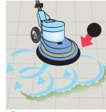
Machine scrub using an overlapping pattern with black stripping pad.
