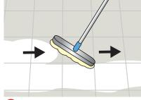
Ensure floor is free from debris/dust before applying a second coat. Apply in opposite direction to the first. Leave a 2.5-5cm gap from the edge.
