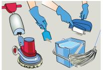
Prepare the floor, remove all traces of old polish/sealer. Ensure floor is clean dry and neutral.
